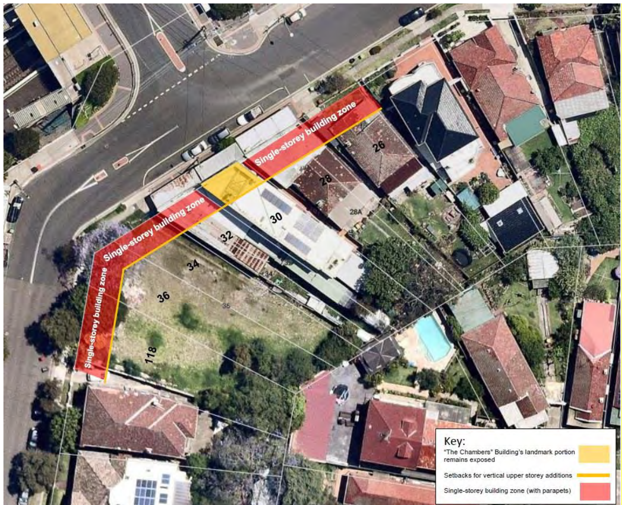
Figure 37: Suggested minimum 6 metres front setbacks to single-storey additions at 26-28 and 32 - 34 Floss Street, and 118 Duntroon Street, Hurlstone Park (indicated by orange line and red shading titled 'Single-storey building zone' (Source: Nearmap 2018)
