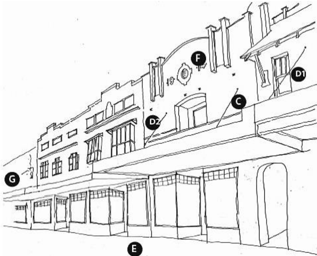
Figure 46: Primary defining elements of a heritage shopfronts including: C) recessed balconies; D1) window patterns, proportions and details; D2) bay windows; E) shopfronts; F) parapets profiles and details; and G) awning alignment, stays, fascias and soffits (Source: Marrickville DCP 2011, Part 5 - Commercial and Mixed-use Development, p.34)
